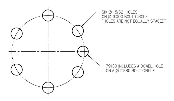
USE AS A PATTERN TO DETERMINE WHICH FLYWHEEL OR DRIVE FLANGE IS NEEDED FOR YOUR ENGINE
