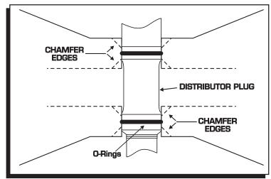
Figure 9 Modified Block for use with O-Rings.
