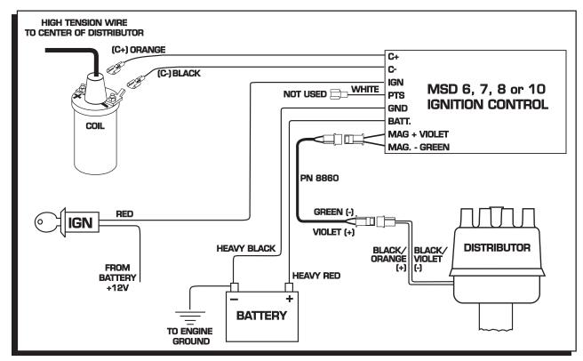
Figure 11 Wiring the Distributor.
