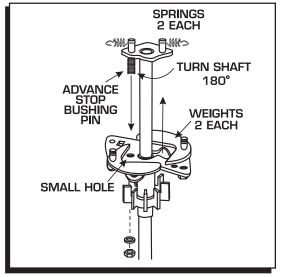
Figure 7 Locking Out the Advance.
