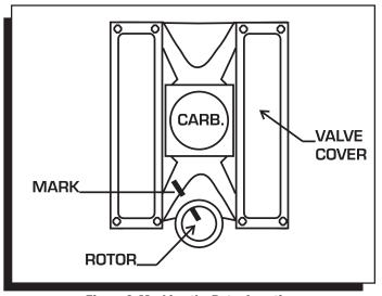
Figure 8 Marking the Rotor Location.
