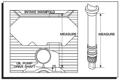
Figure 10 Measuring Oil Pump Shaft Overlap.
