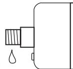
Use Teflon Sealing Tape Or Sealing Compound On Pipe Threads.
