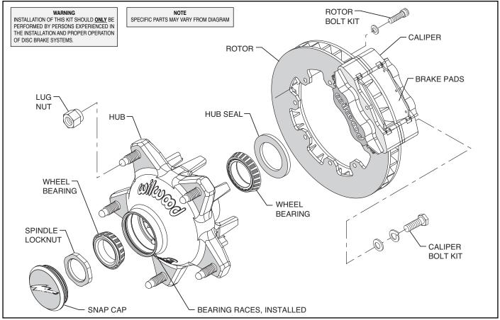
Typical Front Wide 5 Super System Installation Configuration, Major Components Identified
