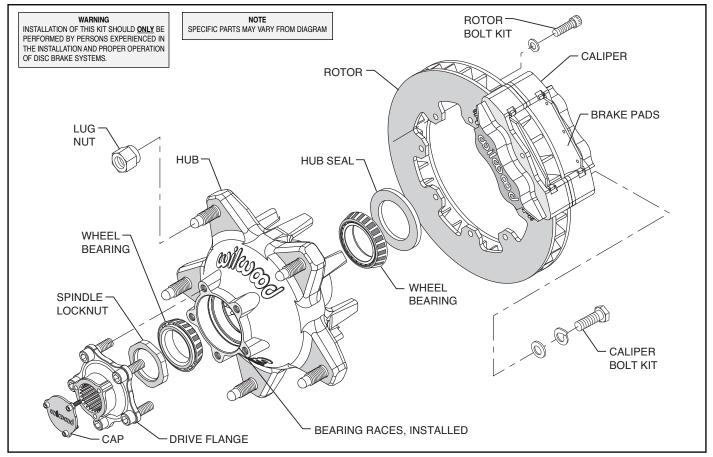
Typical Rear Wide 5 Super System Installation Configuration, Major Components Identified
