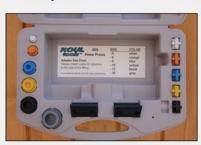
**4)** The chart on the bottom of the case matches the color of the adaptors to the size of the fittings. The adaptors are also marked with the dash numbers. The pinned adaptors are used for angled fittings.
