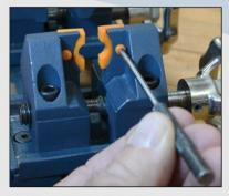
**7)** To remove the adaptors, use a pin punch or similar as shown.
