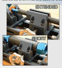
**3)** Extended jaws are for -4 thru -8 hose. Short jaws are for -10 thru -16 hose.
