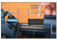
**9)** Clamp the hose in the jaws, leaving enough hose exposed so that the hose can be fully installed on the end of the barb without interfering with the clamp.
