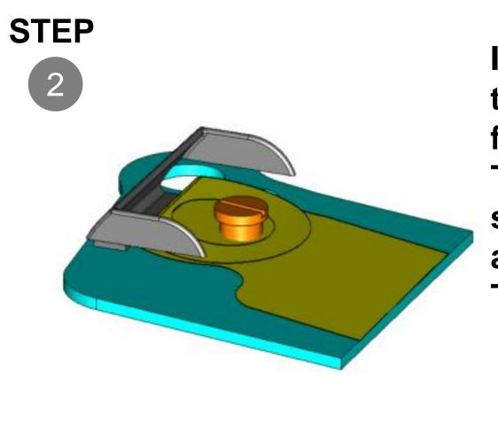
Install tearoffs. Align the EZ Tear with the folded tearoff tabs. The folded stack should be about 1/4" away from the EZ Tear.
