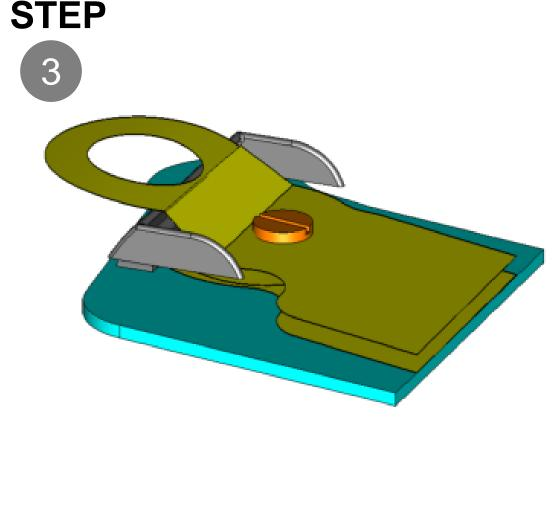
tab to extend over the top of the EZ Tear. Tighten the post to fully secure the EZ Tear. Then rotate and
