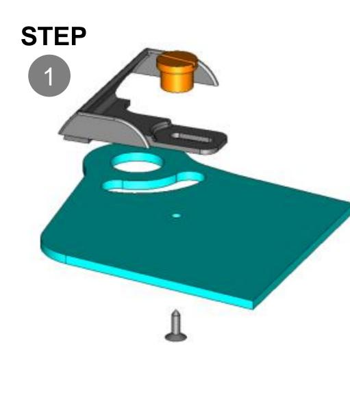
Install EZ Tear beneath the tearoff post. For plastic posts, use the screw provided. If required, trim the base of the EZ Tear to fit your helmet / shield.
