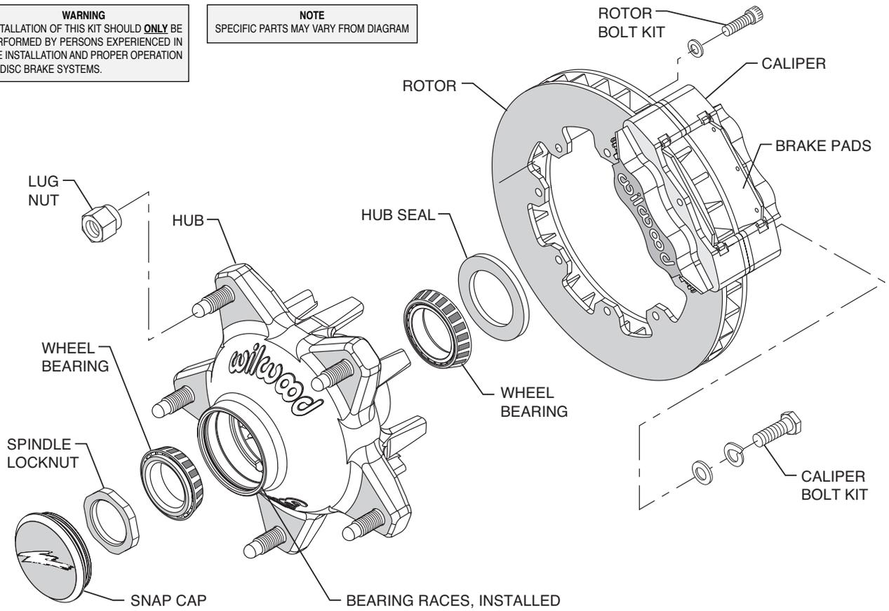
**Typical Front Wide 5 Super System Installation Configuration, Major Components Identified**
