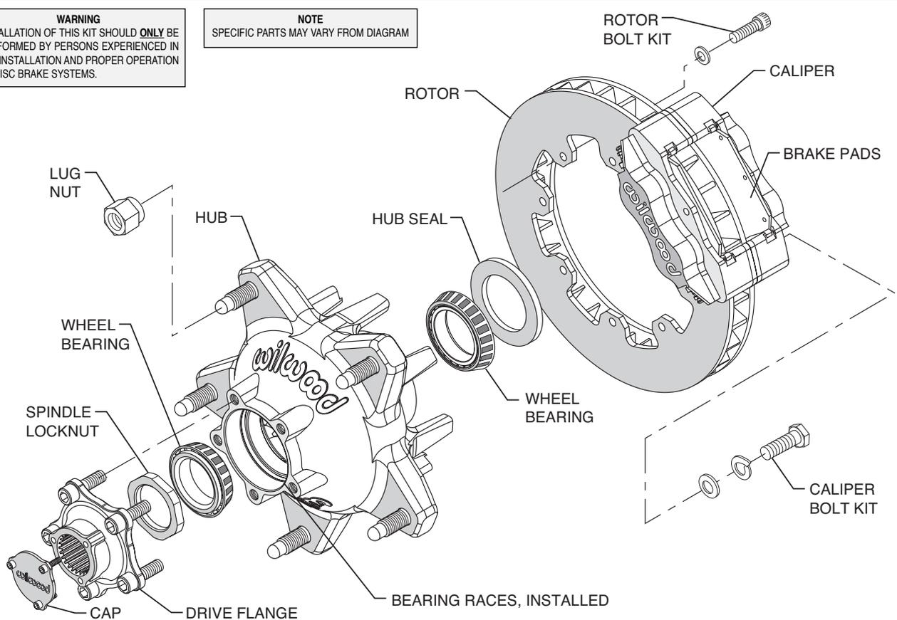
**Typical Rear Wide 5 Super System Installation Configuration, Major Components Identified**
